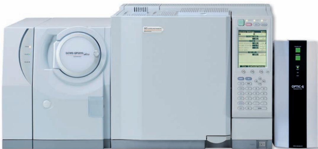
Figure 1: Shimadzu GCMS-QP-2010 Ultra equipped with the OPTIC-4
