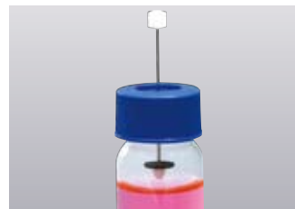
Clean Pin Hole Septum with Vial (40mL) Tighten the septum on the vial.
