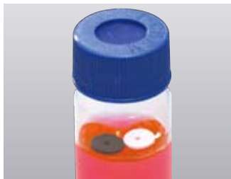
Put the sample into the vial and flow MonoTrap
