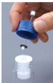
Put the MonoTrap and tighten the septum
