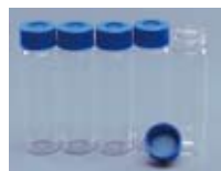
④ Clean Pin Hole Septums with vials (40mL) 5 pcs
