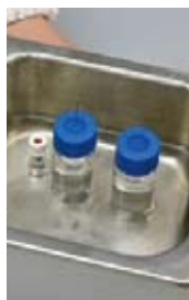
Give it ultrasonic agitation for 5 mins
