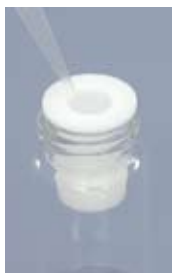
Fill the MT Extract Cup with the extraction solvent
