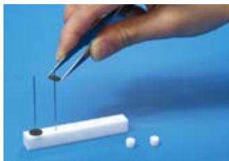
MT Holder & MT Stand Grabs the MonoTrap™ with tweezers and insert the holder into the hole on the MonoTrap™.
