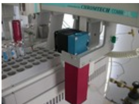
Fig 2: The SPDE - Extraction Cooler is simply mounted on top of a Single Mixer. The SPDE needle penetrates the vial only by a few millimeters.
